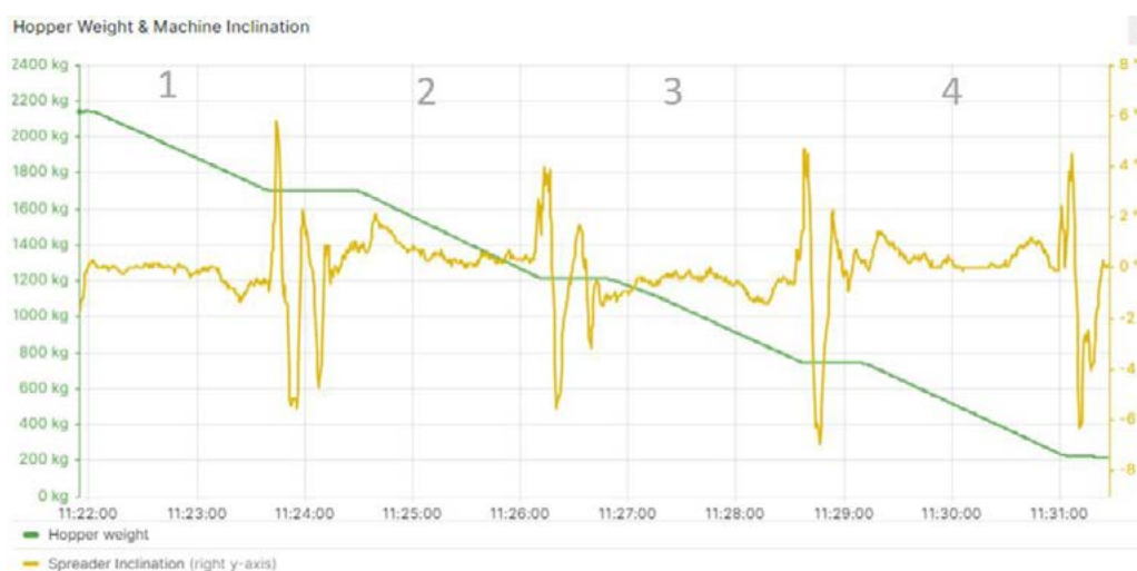
Figure 3.2. Hopper content and spreading inclination as function over time including track number.
