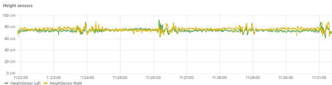
Figure 3.3. Spreader height sensor measurements as function over the time.
