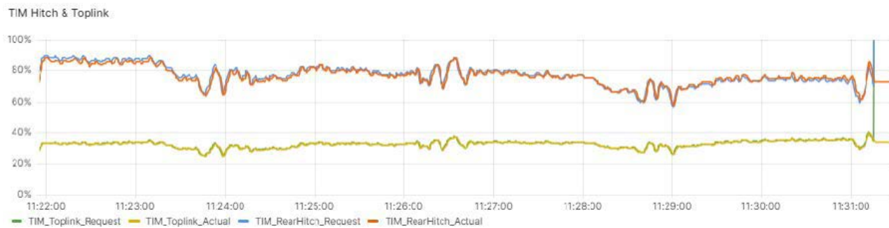
Figure 3.4. Measurements and setpoint for the TIM rear hitch and TIM-like Rear toplink.
