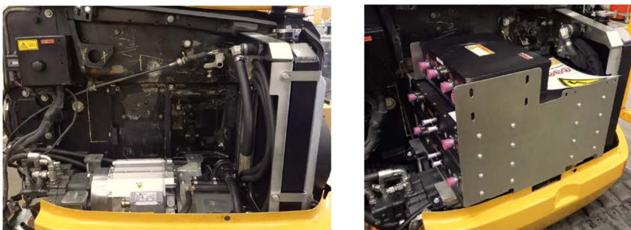
Figure 6. Example of Vensys electric retrofit system integration in machine.
