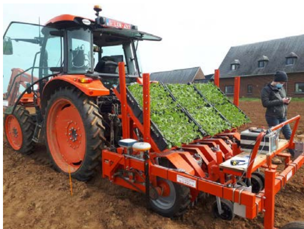
Figure 4. Plantation GPS data acquisition set-up with Sokkia antenna, Septentrio antenna and datalogger.
