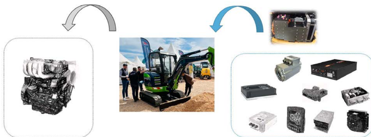
Figure 7. Main component change in the electric retrofit process.
