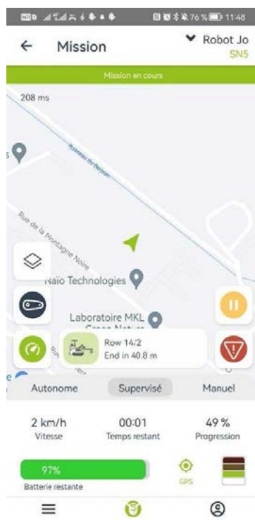
Figure 2. Supervision station giving information about the autonomous mission, and providing restrictive commands like stopping the autonomous operation.
