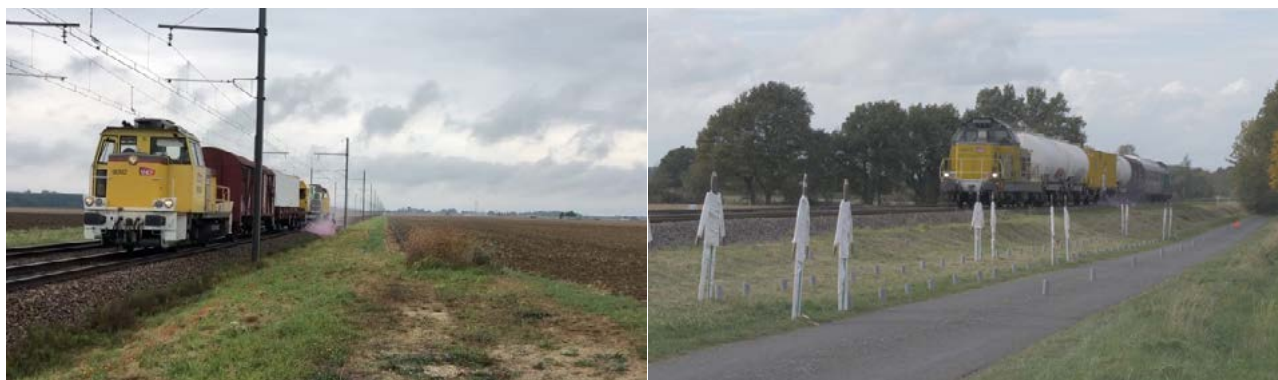
Figure 3. Left: TDR sprayer – right: TDGR sprayer.
