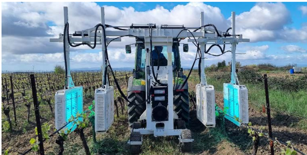
Figure 1. A two-row stimulation system of the UV Boosting company. This system is also suited for full grown grapevine plants.
