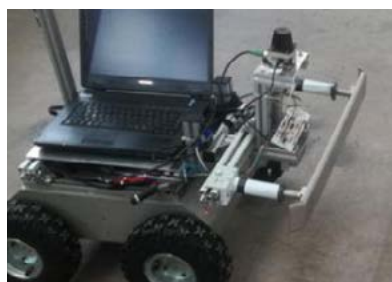
Figure 6. Sensitive bumper probing system mounted on « Effibote3 Robot »
